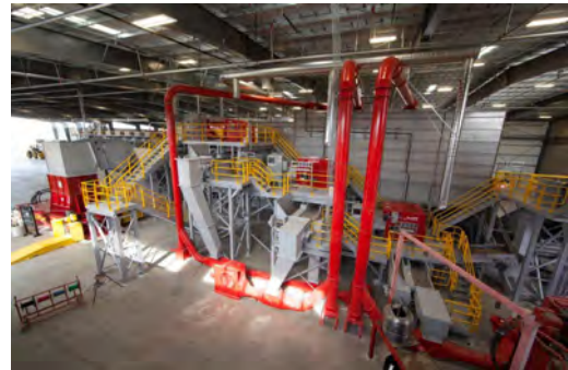
Large Processor or MRF: 90,000 square-foot recovery plant processes up to 30 tons per hour.
