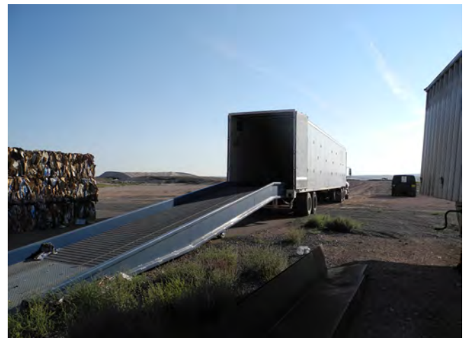
Portable Loading Dock Estancia Valley Regional Recycling Hub
